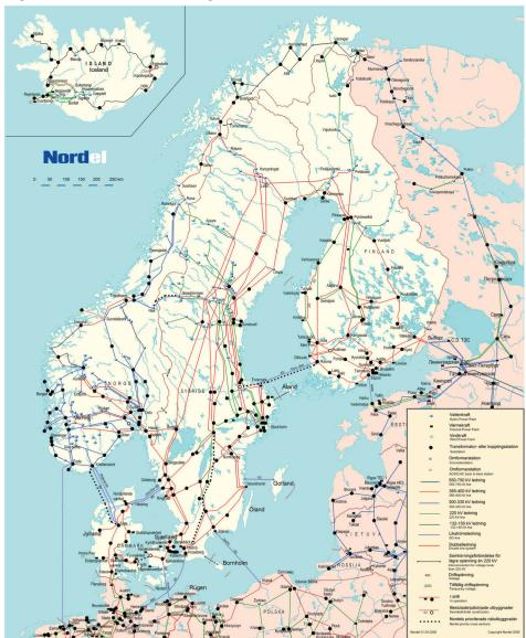
Figure 2.1 The transmission grid in the Nordic countries.
